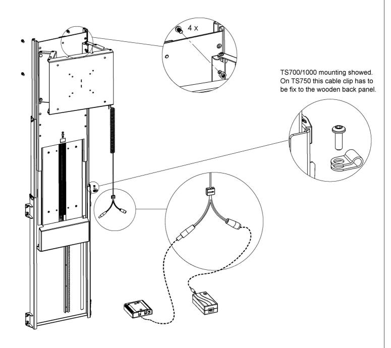
Max allowed weight of TV mounted on SB001: 15 kg/33 lbs Max TV size for SB001 is 46"
