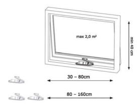
On the frame you need at least 25 mm and on the sill at least 50 mm, when the window is closed.
